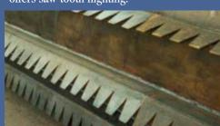
For elongated products (e.g. strands, hay, grass, bagasse) curved, smooth-edged flighting keeps products from hanging up in the flights.
