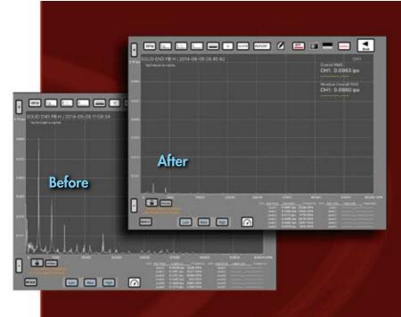
The charts above show vibration amplitude at various frequencies before and after main and motor bearing service.
