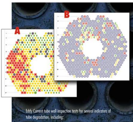
Tube Wall Thinning testing (Chart A) that reveals which tubes show wall loss and to what degree. Similarly, Chart B reports any detected internal pitting, and the severity of pitting, in each tube.
