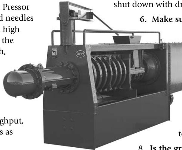
maximum capacity—any wear on the flights and the cage bars will be more even and consistent. When running significantly below maximum, or worse, when empty, all of the components wear unevenly, which in turn will lower a Pressor’s efficiency. Also, always make sure Pressors are properly cleaned at shut down with dry material, then emptied.
