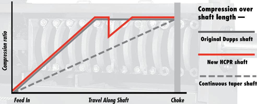
A good time to check to see if you're operating with the most efficient shaft configuration is during machine service. Which brings up another important aspect of press performance, proper maintenance and repair. Shaft flights in particular are susceptible to wear, and can dramatically
