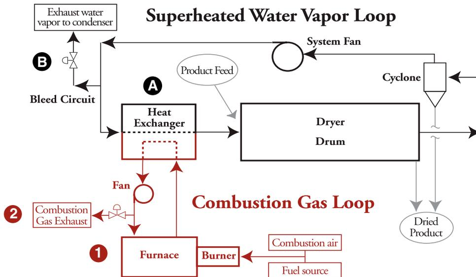
System fan creates a circulating loop of water vapor. Heat is transferred from the heat exchanger (A) to drive the evaporation of moisture from wet feed in the dryer drum. The water evaporated from the feed displaces air in the water vapor loop, creating the “airless” environment. To maintain atmospheric pressure in the dryer, a bleed circuit (B) is needed to exhaust water vapor. This water vapor can be treated with a conventional condensing system or used as a heat source for other processes.
