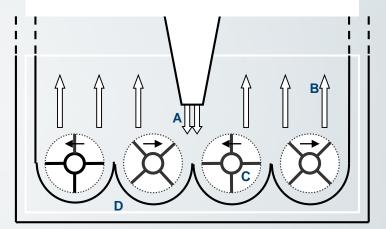
A: Drying gas inB: Drying gas outC: Shaft with paddlesD: Insulated chamber
