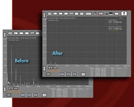
The charts above show vibration amplitude at various frequencies before and after main and motor bearing service.
